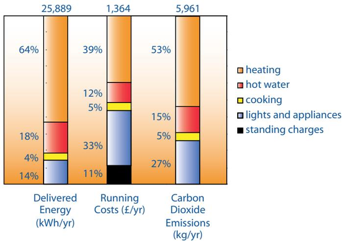
Figure 1.2 The breakdown of annual fuel use, fuel costs and carbon dioxide emissions for a typical 1930s semi-detached house of 90 m<sup>2</sup> floor area
