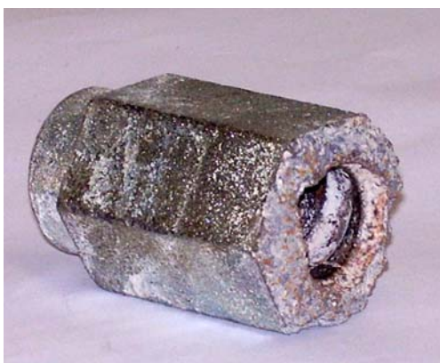
Detail of Failed Connector
